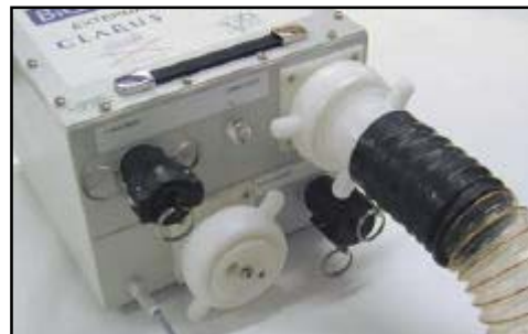
External Catalyst and Pressurisation Unit
